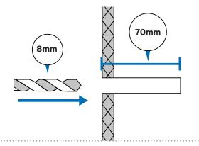
WIRING POWER FOR THE MULTIPLEX UNIT
