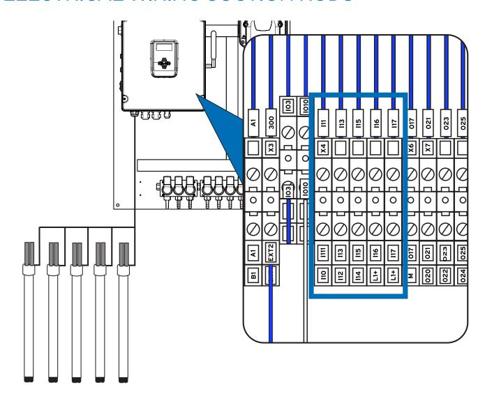
To connect the external suction rods to the machine, utilize inputs I10 to I17, as indicated above.
