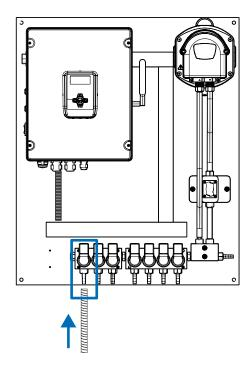
Connect the water supply to the water inlet connection seen on the unit here.
