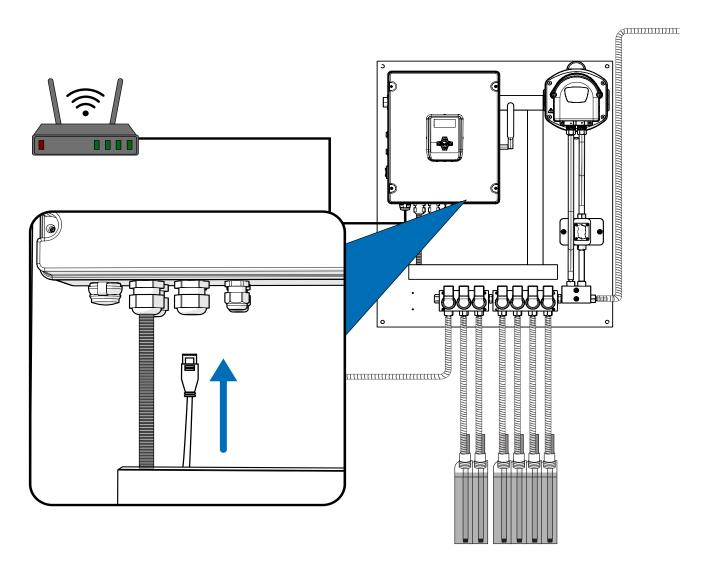
To connect your unit to the internet, simply plug an Ethernet cable into any router through the connector located on the bottom of the main box.
