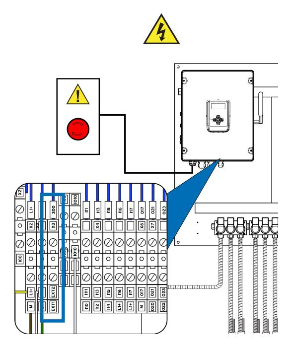
To connect an emergency stop button to your unit, you can use the EXT1 and EXT2 connectors slot shown above.
