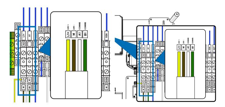
To connect the expansion channel to the unit, connect X2 on the main machine to X1 on the expansion channel.
