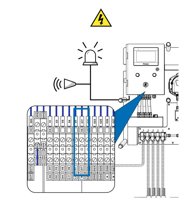
To connect an external alarm or warning light to the system, utilize slot X6 as depicted above.
