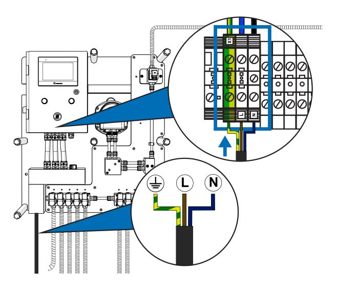
For the power supply of the equipment you must use **3x1'5mm2 cable**. Insert the cable through the channel located at the bottom left and use one of the cable glands to insert it safely inside the control cabinet. Connect to the terminals identified with **X1** found on the lower left of the connections.
