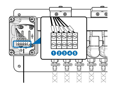
Use a **7x1mm^2** cable for the connection between the control cab inlet and the distributor. Connect the distributor to terminal block **X7**. Each terminal connection corresponds to the outlets numbered from left to right, with the number dependent on the order. Below is the wiring diagram for the main unit.
