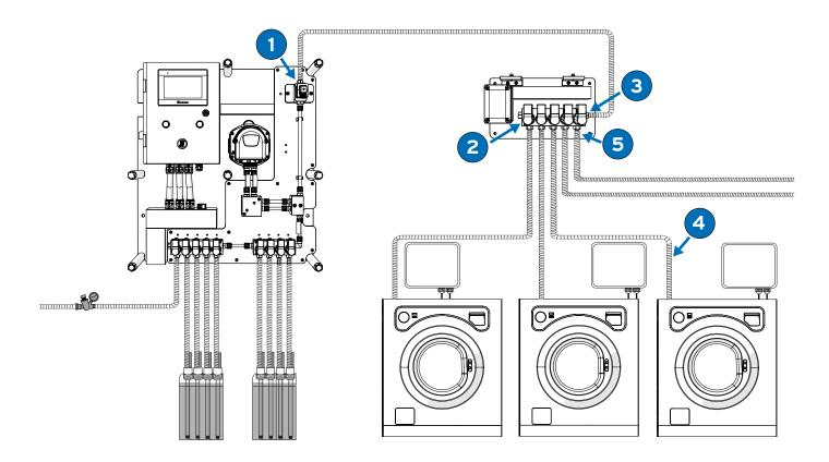
To connect equipment, distributor and washers, use 10x16 mesh PVC pipe and stainless steel clamps.
