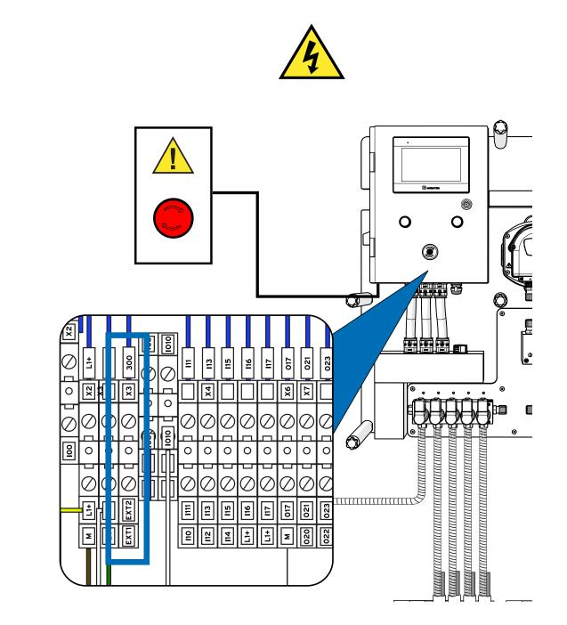
To connect an emergency stop button to your unit, you can use the EXT1 and EXT2 connectors slot shown above in series.
